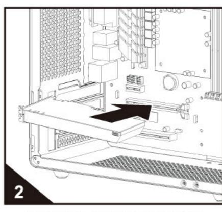
Insert VGA card into the slot of M/B according to the arrow direction
