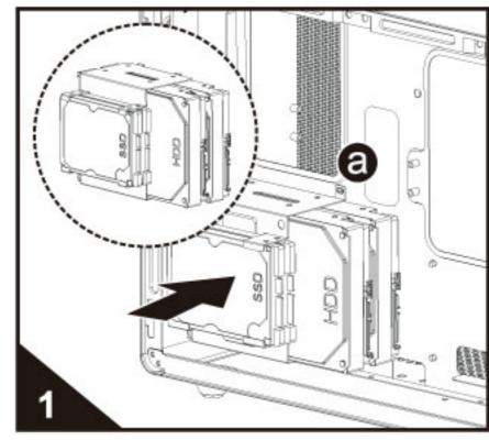
HDD/SSD cage can be installed with HDDx2 + SSDx2
