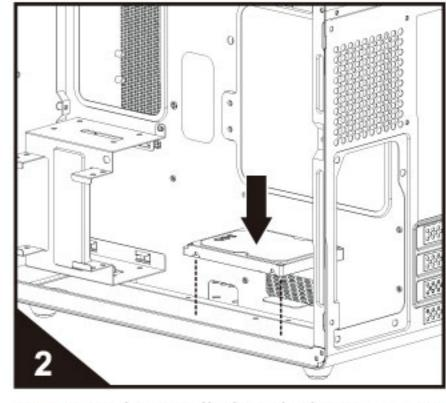
SSDx1 can be installed on the bottom cover
