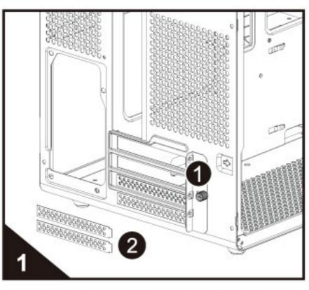
Unscrew the screws fixed PCI slot covers, then break off PCI slot cover
